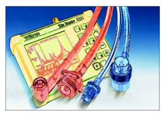
This range of test leads has been specially designed for adverse outdoor applications using the SiteMaster measurement unit series from Anritsu. The waterproof test leads are all provided with a ruggedization consisting of a steel spiral and a resistant PUR jacket, which protects the coaxial cable against mechanical stresses such as compression and tension. Despite this ruggedization, the cable remains astonishingly flexible, offering users agreeable ease of handling.
